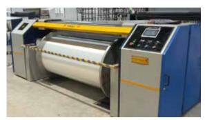
Amritlakshmi's Hydraulically operated Direct Warper with Magazine Creel along with Yarn Eveniser to stabilize the Yarn sheet can give High Production at High Quality.
